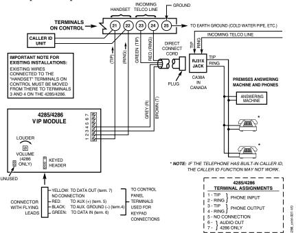
Figure 13. 4285/4286 Phone Module Wiring Connections
